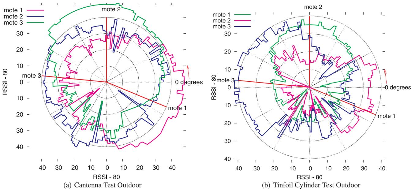
Figure 7. Outdoor tests: Multiple nodes
