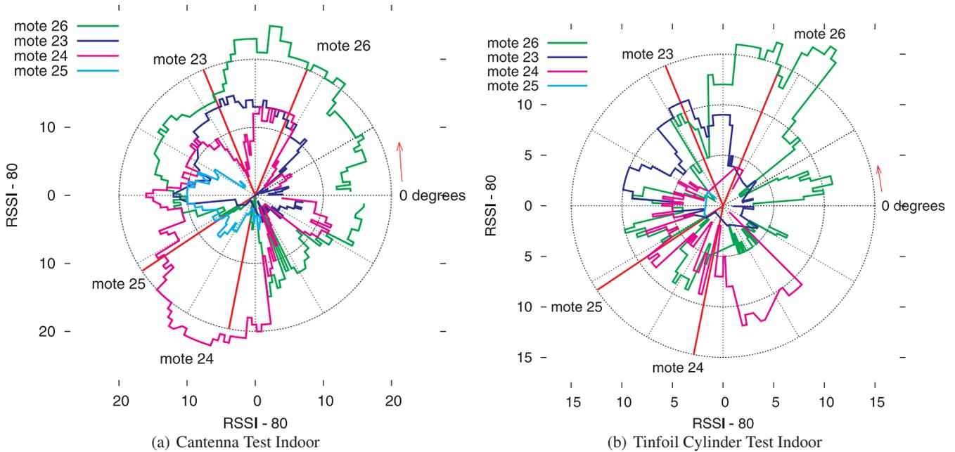
Figure 6. Indoor tests with multiple motes
