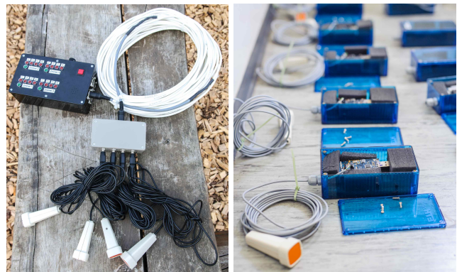
Figure 1: Old wired system with control light panel (left) and new TelosB-based system (right).
